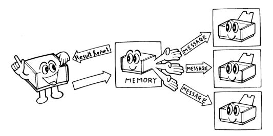
The message is stored in the memory of the broadcasting transmitter and transmitted to each designated receiver sequentially.
